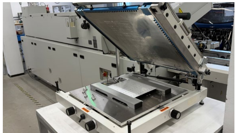
The solder paste printer applies solder paste precisely to the PCB, ensuring clean and reliable SMD solder joints.
