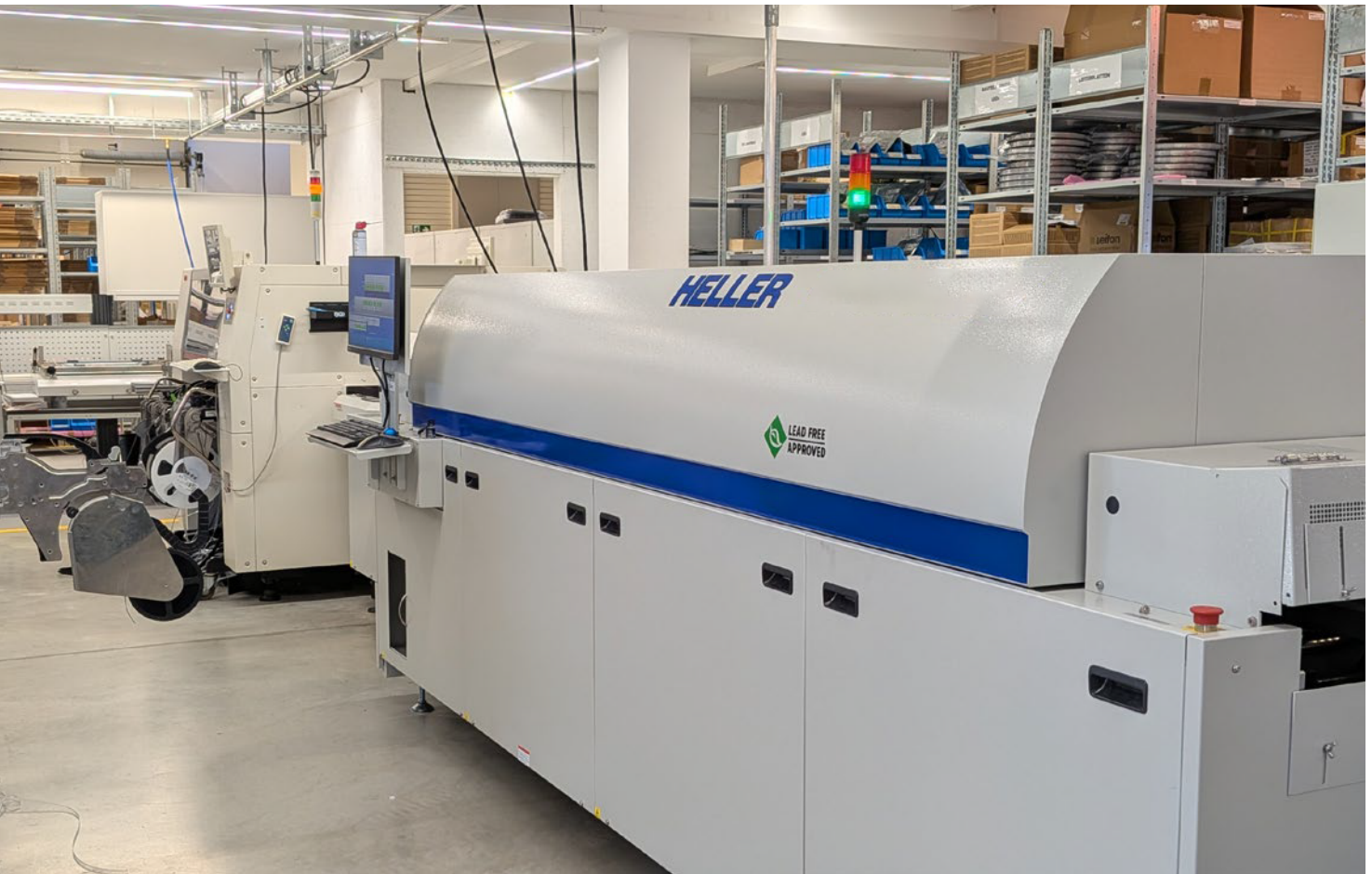
The reflow oven melts the solder paste and creates stable SMD solder connections.
